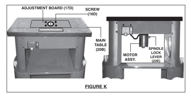
2. **NOTE:** The height of the Adjustment Board (17D) can be adjusted by inserting a hex wrench (not included) through the Adjustment Board and adjusting each Hex Screw (23B) individually. Once adjusted, secure the Adjustment Board to the Main Table (20B) with four Screws (16D). **(See Figures J and K.)**
